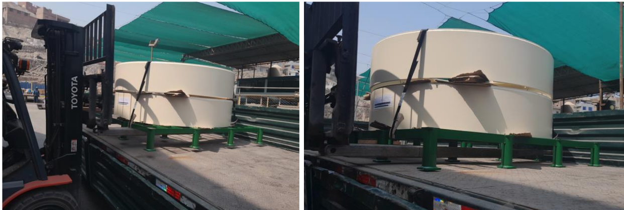
Figures 20 & 21. Steel pallet handling with forklift.
