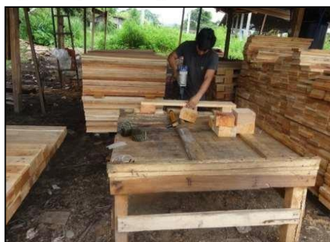
Figure 3. Backcutting, cutting diagram, sawing, and assembling of pallets.
