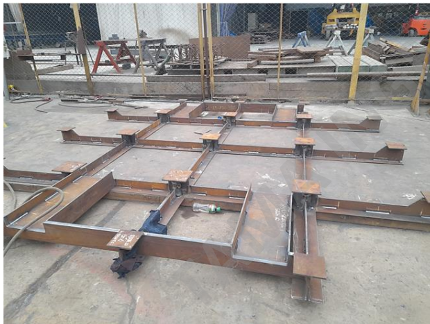
Figure 18. Design of metal pallets made from scrap steel.
